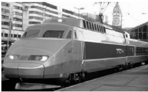
TGV Sud-Est Fleet: 110 First service: 1981 Output: 6420 kW Catenary design: 25 kV/50 Hz + 1500 Vdc + 15 kV/16.7 Hz Train protection systems: TVM 300/TVM 430 + KVB *Renovations in 1996 and 1999
