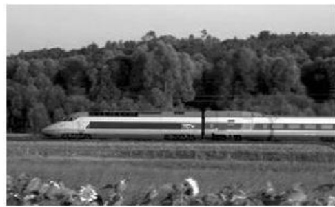
TGV Atlantique Fleet: 105 First service: 1989 Output: 8800 kW Catenary design: 25 kV/50 Hz + 1500 Vdc Train protection systems: TVM 300/TVM 430 + KVB
