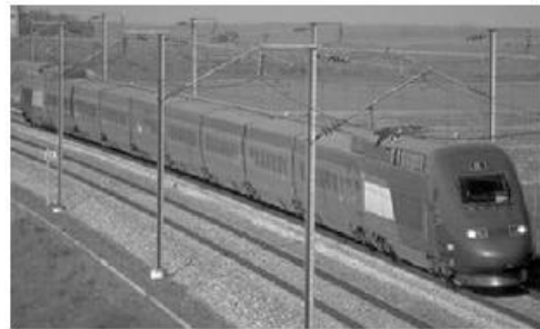
Thalys Fleet: 17 First service: 1996 Output: 8800 kW Catenary design: 25 kV/50 Hz + 1500 Vdc + 15 kV/16.7 Hz + 3000 Vdc Train protection systems: TVM 430 + KVB + TBL + ATB + Indusi + LZB * 6 SNCF, 7 SNCB, 2 NS and 2 DB AG
