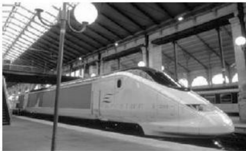
Eurostar Fleet: 31 First service: 1994 Output: 12,240 kW Catenary design: 750 Vdc + 25 kV/50 Hz + 3000 Vdc Train protection systems: AWS/TPWS + TVM 430 + KVB + TBL * 16 SNCF, 4 SNCB and 11 BR
