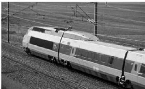
TGV Réseau Fleet: 89 First service: 1993 Output: 8800 kW Catenary design: 25 kV/50 Hz + 1500 Vdc + 15 kV/16.7 Hz Train protection systems: TVM 430 + KVB + TBL + ATB + R54 * Of which 10 PBA
