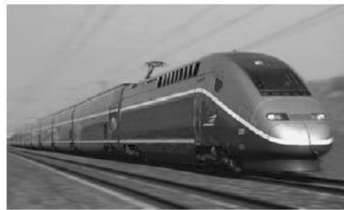
TGV Duplex Fleet: 36 First service: 1996 Output: 8800 kW Catenary design: 25 kV/50 Hz + 1500 Vdc Train protection systems: TVM 430 + KVB
